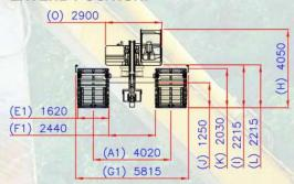
BASE MACHINE TOTAL WEIGHT FLOAT CAPACITY 20 TON CLASS 32000 Kg 40 m3
